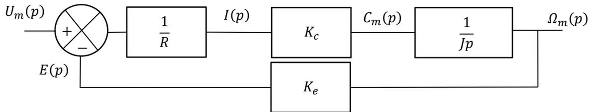
$$H_m(p) = \frac{\Omega_m(p)}{U_m(p)} = \frac{\frac{K_c}{RJp}}{1 + \frac{K_e K_c}{RJp}} = \frac{K_c}{RJp + K_e K_c} = \frac{\frac{1}{K_e}}{1 + \frac{RJ}{K_e K_c} p} = \frac{K_m}{1 + T_m p} \quad ; \quad \begin{cases} K_m = \frac{1}{K_e} \\ T_m = \frac{RJ}{K_e K_c} \end{cases}$$
